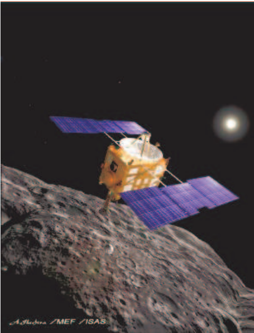
Artist's conception of the Hayabusa spacecraft deploying one of the surface target markers that will be used to guide the spacecraft's descent to the surface of asteroid Itokawa.
