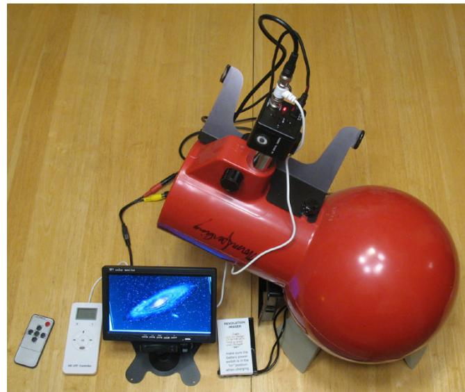
The Revolution 2 imager on an Astroscan, showing an image of a calendar photo of M31 on the other side of the house.
