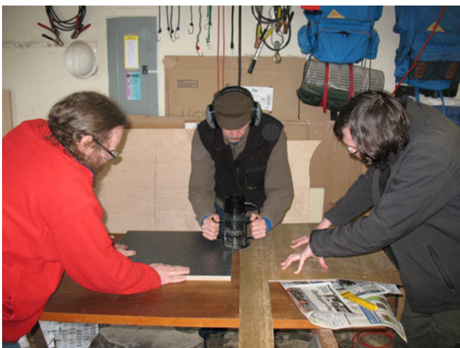
Andy and Galen hold the pieces while Randy trims the formica on the azimuth bearing
