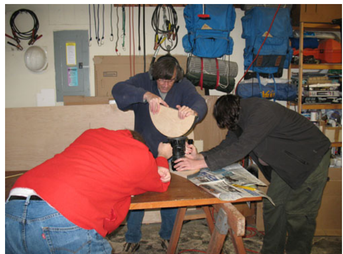
Andy and Galen hold the router while Jerry trims the formica on the altitude bearing
