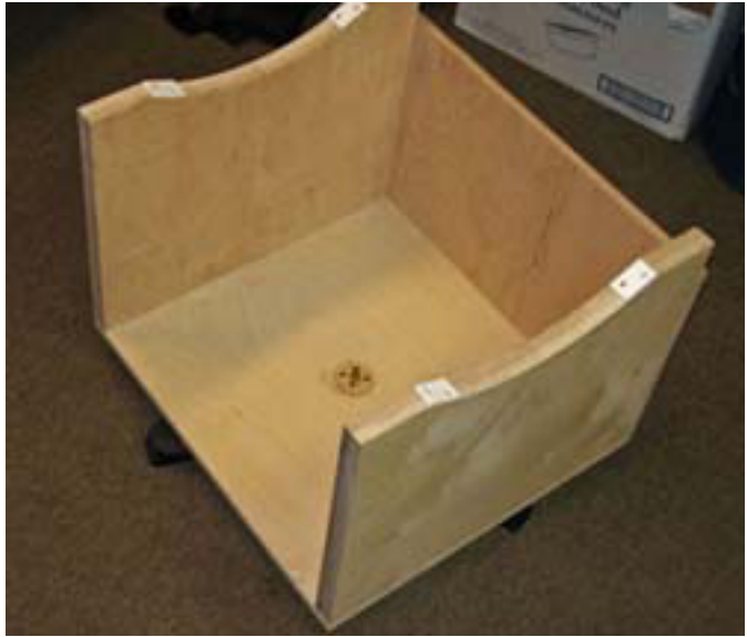
Rocker box (will be shortened and lightened once balance point of scope is known.)
